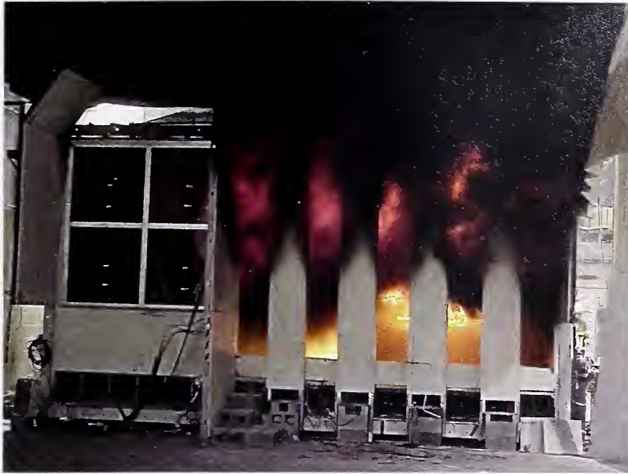
Figure 6–34. Three-workstation fire test, 2 min after the start.
