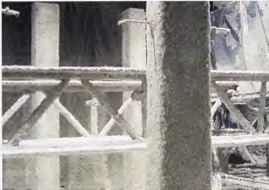
Figure 6-42. SFRM-coated steel components prior to a test.
