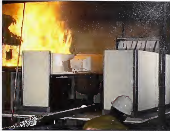
Figure 6–31. Fire test of a single workstation.
