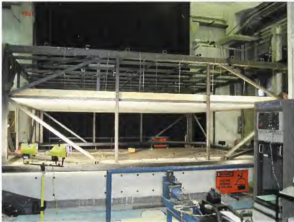
Figure 6–29. Ceiling tile system mounted on the shaking table.
